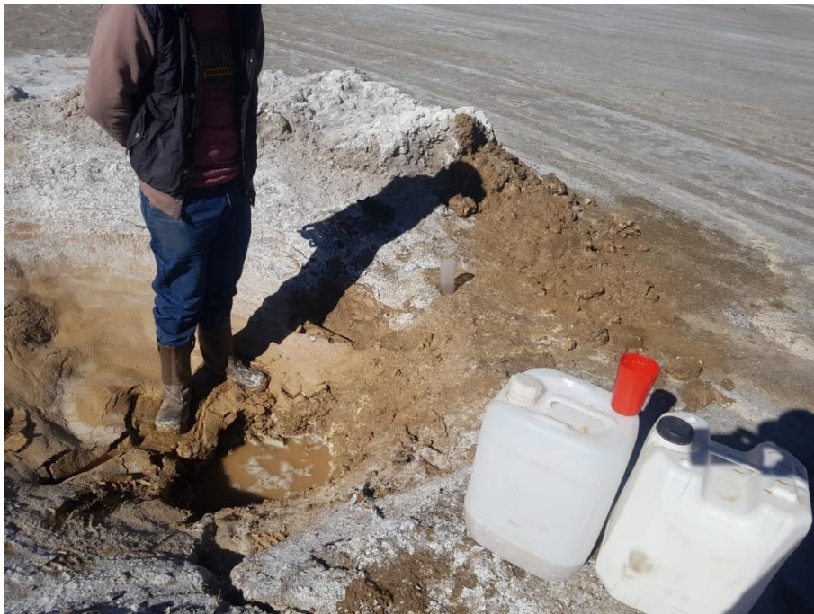
Figure 1. Extraction well from where the brine was extracted and sampled after settling
