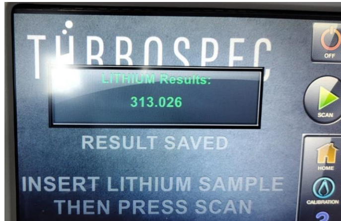
Figure 2. Assay of one of the four samples showing 313.026 ppm lithium
