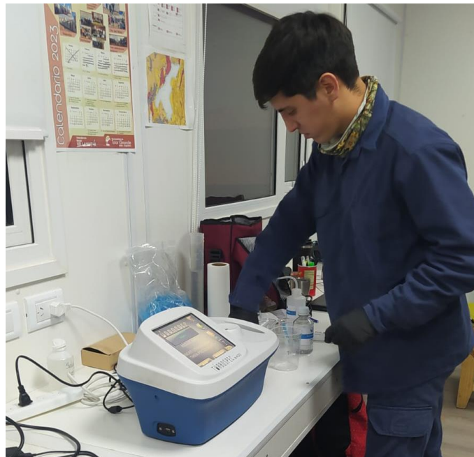
Figure 3. Chemical analyst using the TurboSpec E400 lithium assay machine on Patagonia Lithium brines
