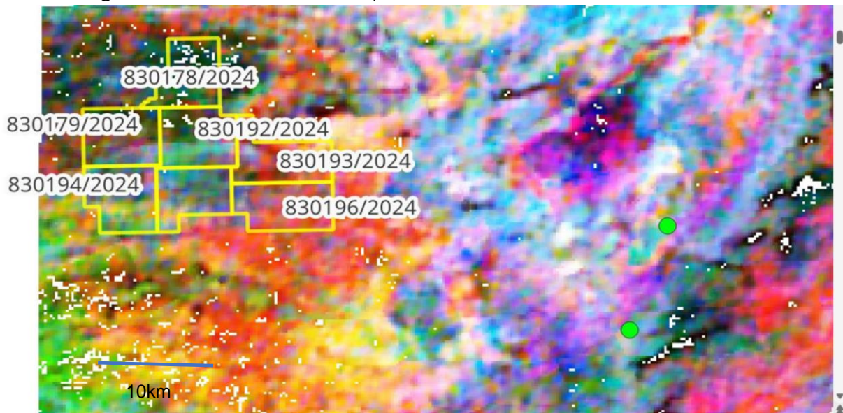
Figure 1. 830178 and other concession applications are shown. Green dots are where REE have been found. The radiographic map shows uranium in green, thorium in blue, fenitization in white. We will target the green and blue areas for REE ionic clays.
