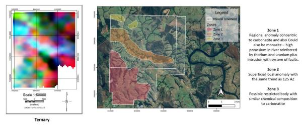
Figure 3. Shows the three zones in the Goais project we have targeted, zone 1 in south with strong radiometric anomaly and system of faults.
