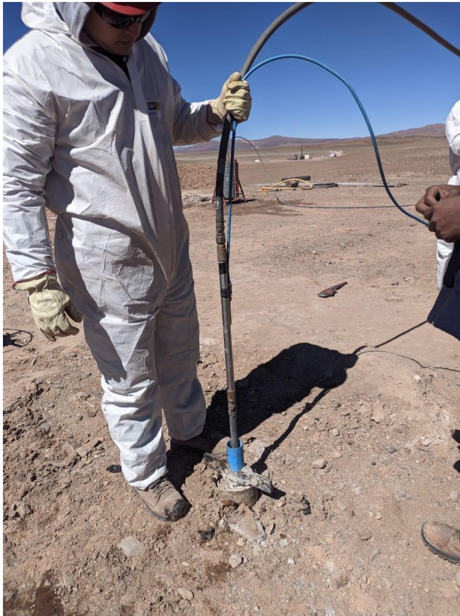
Figure 2. Operator holding 105m suction hose with Jam 24-02 well in background.
