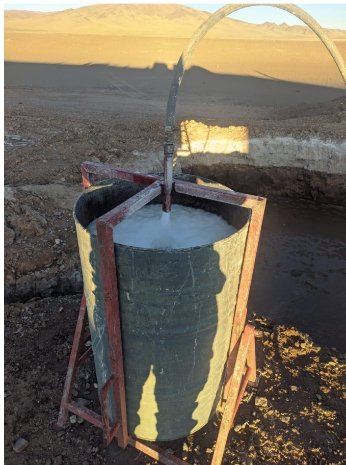
Figure 1. Brines being extracted from the well JAM 24-01 – a total of 25 x 200L drums
