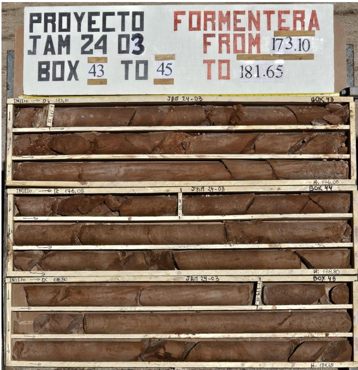
Figure 2. Porous sandy clay matrix where highest flow rate to date was achieved.
