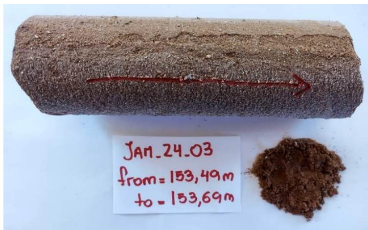
Figure 3. Core sample showing porous sandy clay matrix where highest flow rate was achieved to be tested.
