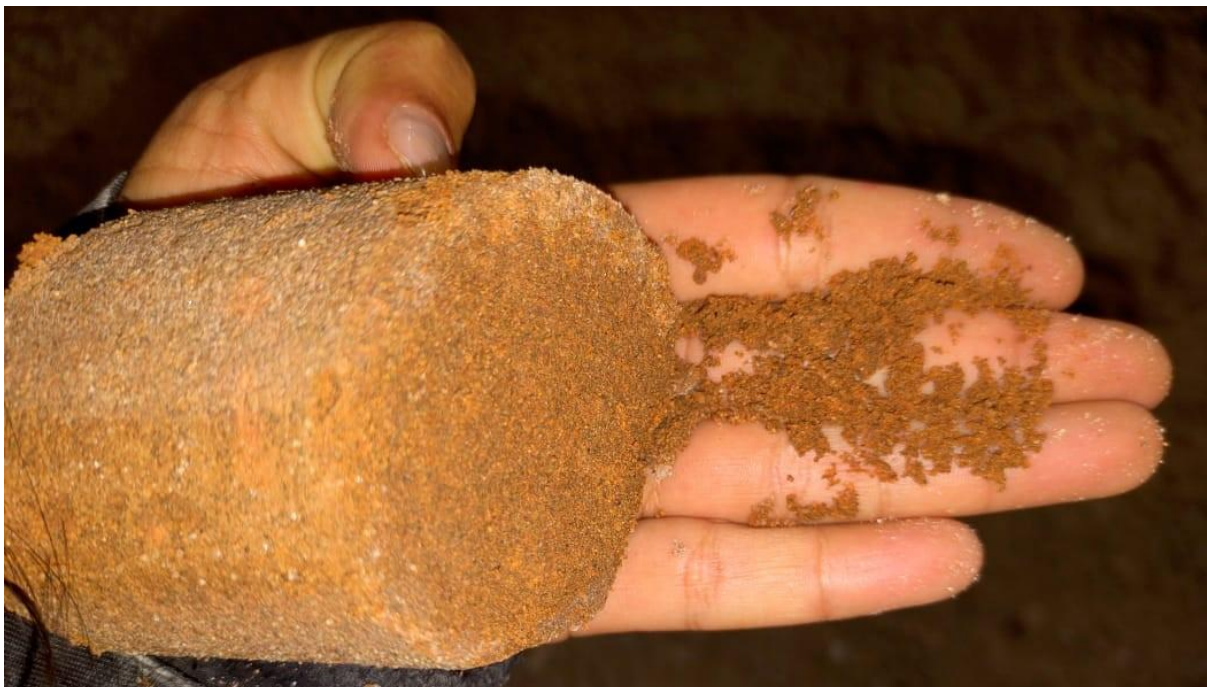
Figure 1. Core from 152m showing friable, high porosity sandstone holding brine
